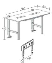
Seat size: 960 mm x 400 mm seat with 100 mm x 60 mm coved plated rear legs for fixing to floor with 10 mm front leg Acetyl plugs to suit shower cubical gradient.
